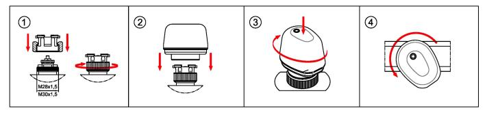
Remove the withe cap on the valve or on the insert of the manifold bar. Install the quickcoupling system on the insert and screw the ring to its end. Tighten the actuator on the locking nut with the aid of the dowels. While holding down the actuator towards the quickcoupling system, turn it clockwise until it stops
