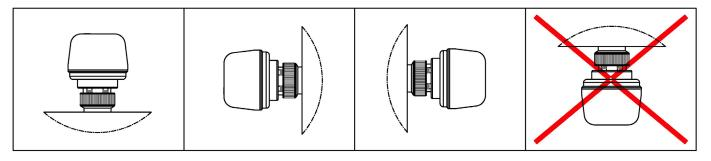
We recommend installing the electrothermic actuators in a horizontal or vertical position, never overturned! Possible condensation on valves and manifolds could reach and damage the actuator.
